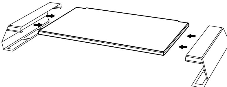
5. Place the cover on the grill grates so that the **outer burners are positioned directly under the gap** between the side panels and the narrower pizza stone, which you place in the centre at the bottom. The **centre burner** is then located **centrally** under the pizza stone.
