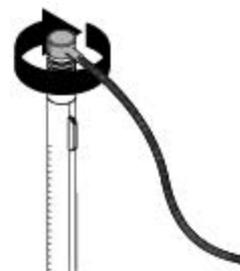
11. Insert a burner tube through the hole located in the front panel so that the gas hose is on the outside and facing towards you. Insert the burner tube at a right angle, and make sure that the fin points upwards.
