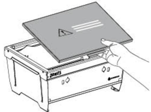
5. Turn the grease drip tray over so the handle is facing up.
